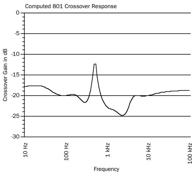
**Note that this is the calculated crossover response, not the loudspeaker response.** Obviously the relative efficiency and the real world frequency response of the driv-
