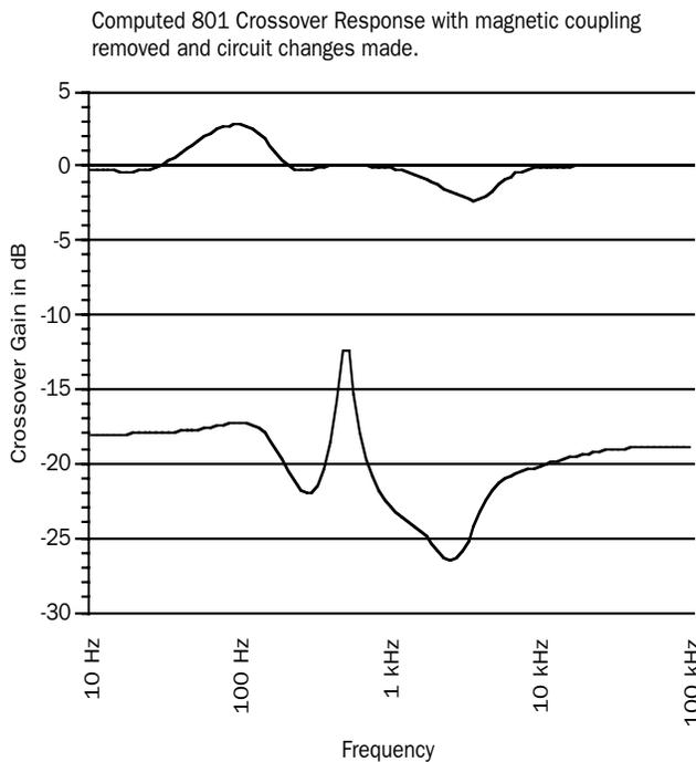
Note that this circuit change has done several things. First the bass drive is much smoother and overall stronger. Second, the drive to the midrange speaker is less peaky. Third, the drive to the tweeter is smoother, and slightly reduced. The following graph shows the calculated stock drive (taking the undesirable magnetic coupling into consideration) in black and shows the calculated crossover frequency response after all fixes in grey.
